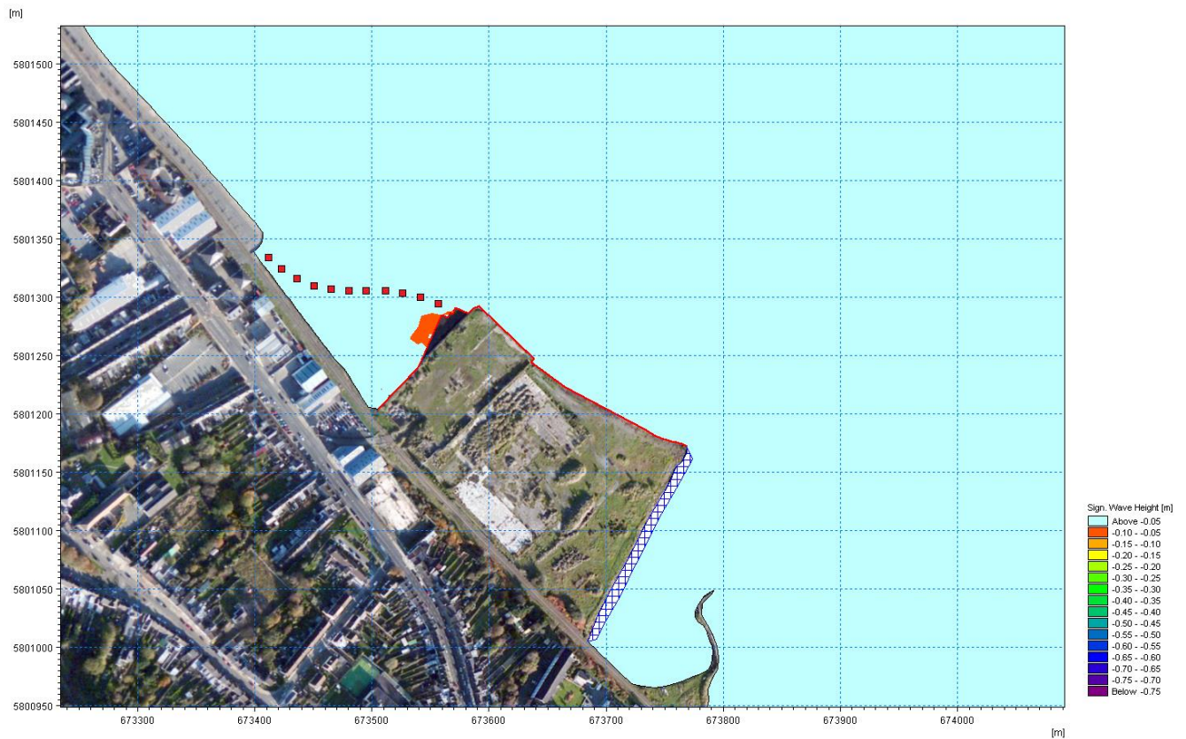
Figure 11: Difference in 1 in 200 year north easterly storm wave climates – Proposed Trinity Wharf Development without marina in situ (proposed minus existing).
